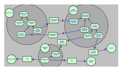
Fig. 9. Structure of the Agent Authenticator pattern.
