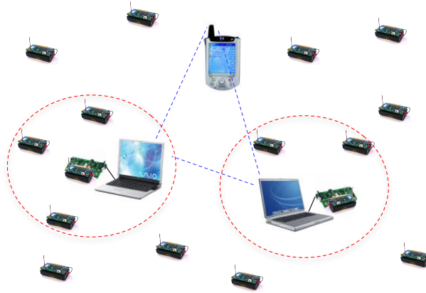
Fig. 2. Operational scenario showing one hop communication between base stations (laptops) and sensors and multi-hop communication among base stations and clients (PDAs). Client agents can also be co-located with the base stations (e.g., running on the laptops).
