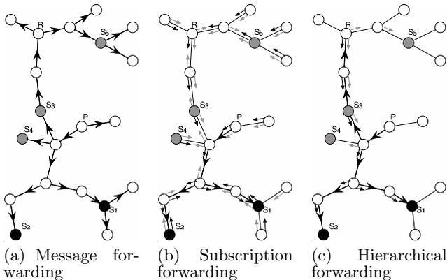
**Figure 1: Tree-based routing strategies.** Broker  $S_1$  and  $S_2$  subscribed (through their clients, not shown in the figure) to the same “black” filter, while  $S_3$  subscribed to “gray”. Arrows represent the content of subscription tables for the filters of the same color. Broker  $P$  published a message matching the black filter but not the gray one. The path followed by this message is shown by thick arrows. Broker  $R$  is the root for hierarchical forwarding.
