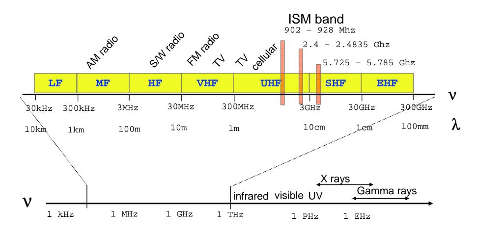
Propagation characteristics are different in each frequency band
