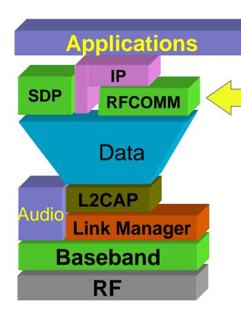
Serial Port emulation on top of a packet oriented link
