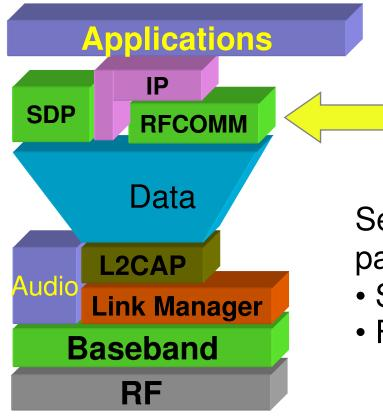
Serial Port emulation on top of a packet oriented link
