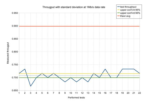
Figure 4: Line chart of the 22 measurements for the 1Mb/s data rate case with mean, upper and lower interval for 95% confidence
