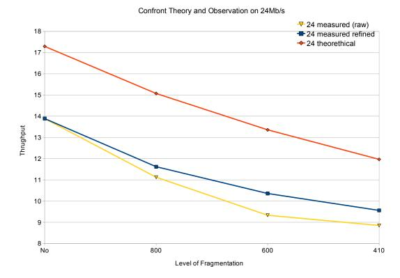
Figure 9: comparison of theoretical, measured and refined throughput in relation to the fragmentation threshold for speed 24 Mb/s
