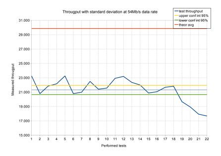
Figure 11: Line chart of the 22 measurements for the 54 Mb/s
