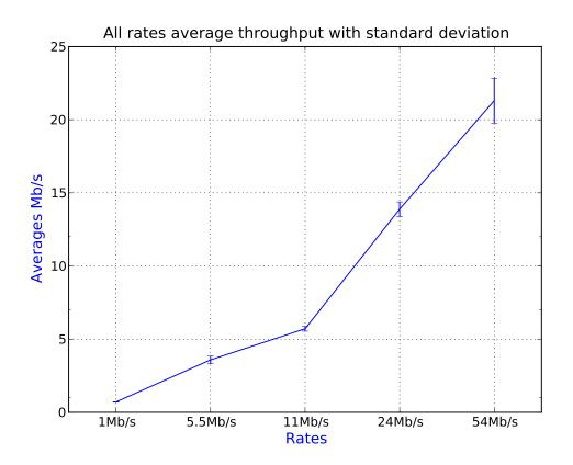
Figure 3: Average of all the tests average throughput for all rates. The error lines represent the standard deviation for each tested rate
