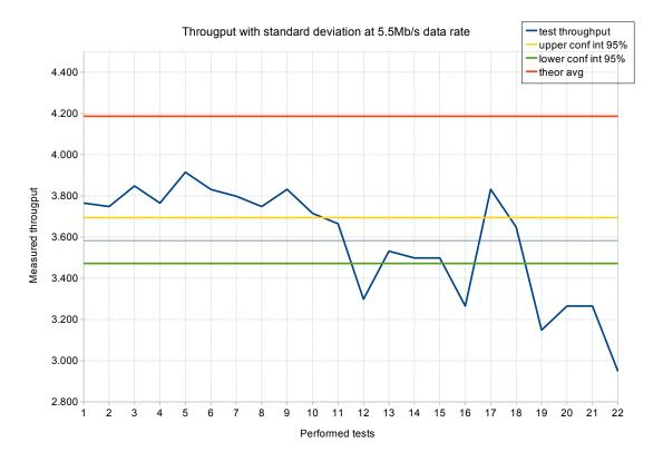
Figure 5: Line chart of the 22 measurements for the 5.5Mb/s rate case with mean and upper and lower interval for 95% confidence
