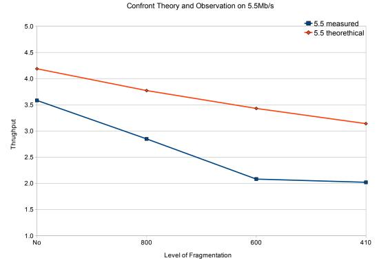
Figure 8: comparison of theoretical and measured throughput relative to the fragmentation threshold for 5.5Mb/s datarate
