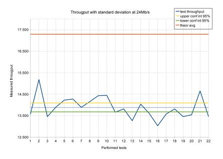
Figure 10: Line chart of the 22 measurements for the 24 Mb/s
