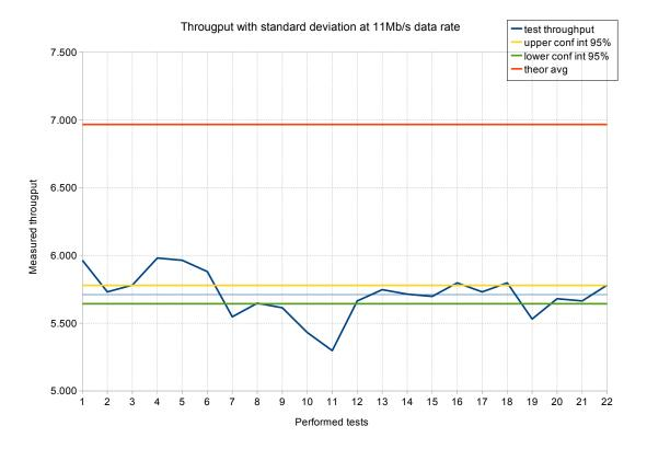
Figure 6: Line chart of the 22 measurements for the 11Mb/s rate case with mean and upper and lower interval for 95% confidence
