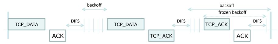
T<sub>c</sub>=2 TCP\_DATA+3 SIFS+3 DIFS+2 TCP\_ACK+2 ACK+2 E[backoff]
