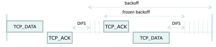
T<sub>b</sub>=2 TCP\_DATA+2 SIFS+2 DIFS+2 TCP\_ACK+ACK+E[backoff]
