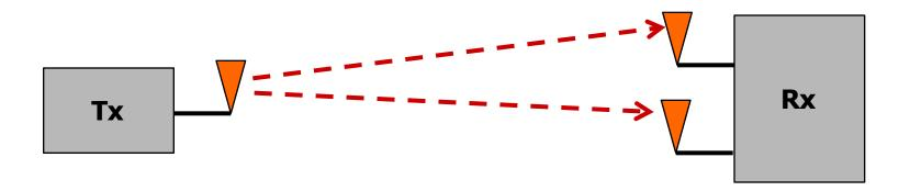
The phase of the signal to single antennas is controlled to obtain constructive interference in the desired direction
