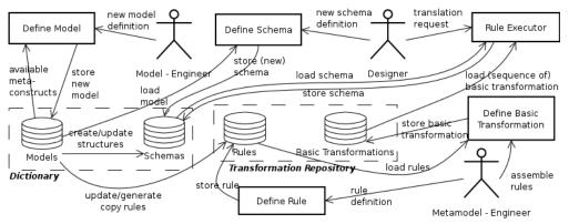
Figure 1: a sketch of the architecture of ModelGen
