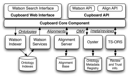
Fig. 2. Cupboard's architecture.
