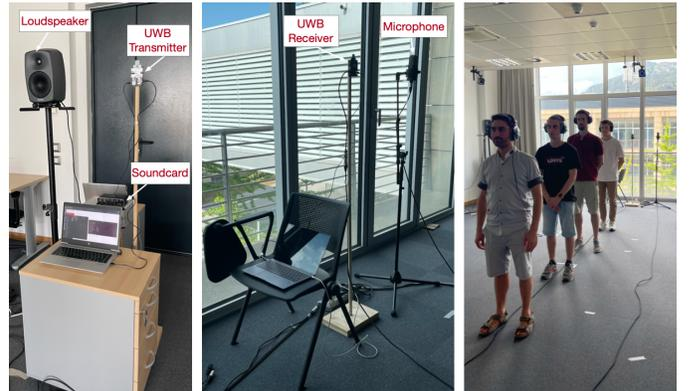
Fig. 3. Transmitter (left) and receiver (middle) apparati; NLOS setup (right).
