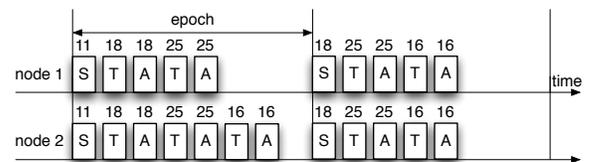
**Figure 5: Channel hopping in CRYSTAL.** The number on each CRYSTAL phase denotes the channel used.
