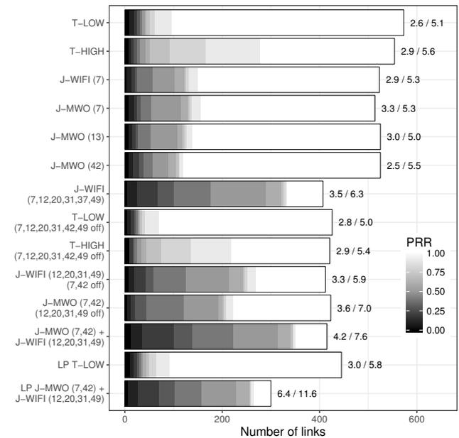
**Figure 4: Link quality distribution (PRR) and network radius (mean/max) in various interference scenarios.**
