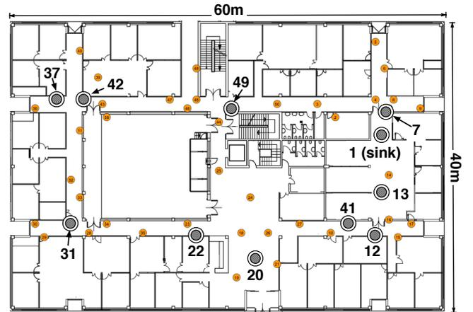
**Figure 2: Position of the jammers in the testbed.**
