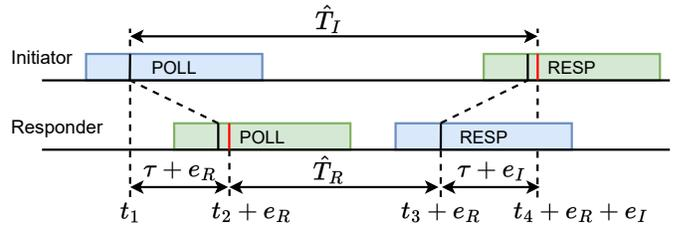
Fig. 1. Single-sided two-way ranging.
