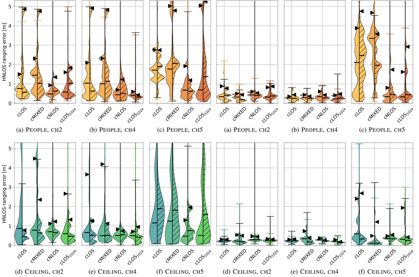
Fig. 4. CORRIDOR: Ranging errors in HNLOS. Violins show R-SHIELDED (left) and I-SHIELDED (right); whiskers show the extremes (dark for I-SHIELDED); inner ticks show the median  $\mu$ ; triangles show the 90<sup>th</sup> percentile.
