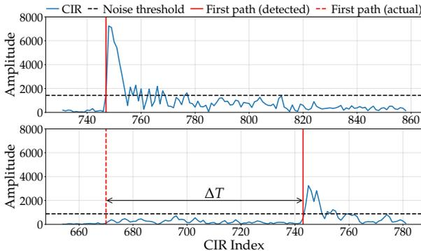
Fig. 2. In LOS (top), the first path is correctly detected from the CIR. In HNLOS (bottom), it is severely attenuated by body occlusion, causing a later reflection to be detected instead.
