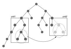
**Fig. 2.** A hierarchical data structure where units in range agree to transfer a subtree that is under their jurisdiction even though parts of the global structure remain hidden. Moving a subtree distributes data to a different location to satisfy changing access patterns.
