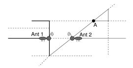
Fig. 3. Ant 1 learns from Ant 2 about landmark A when, by virtue of being in range, the locally built maps are merged. Solid lines denote paths explored by Ants 1 and 2, and dashed lines denote unexplored regions. After sharing, each ant has the same knowledge of the global structure.
